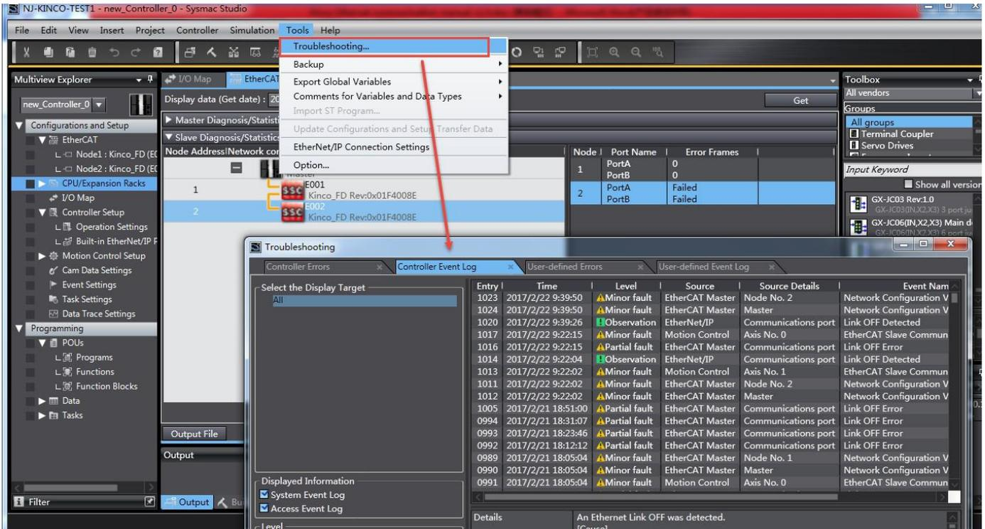
Or at I/O Map frame, if see value which is read from slave stations, it means communication successful.
