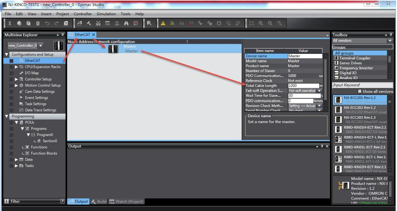
Find Kinco\_FD in toolbox and right click to insert slave station of Kinco servo (insert the pieces that you real use). After inserted, the slave stations will be shown in Network configuration interface and distributed the address automatically.
