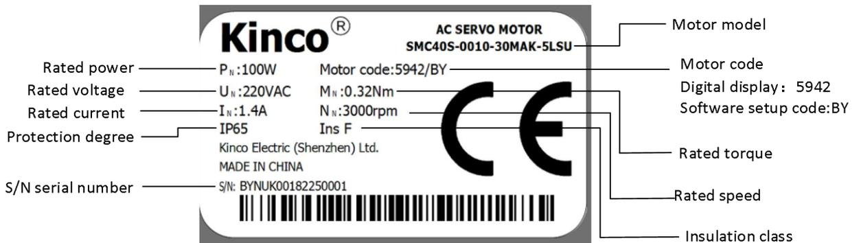
Figure 1-4 Motor nameplate description
