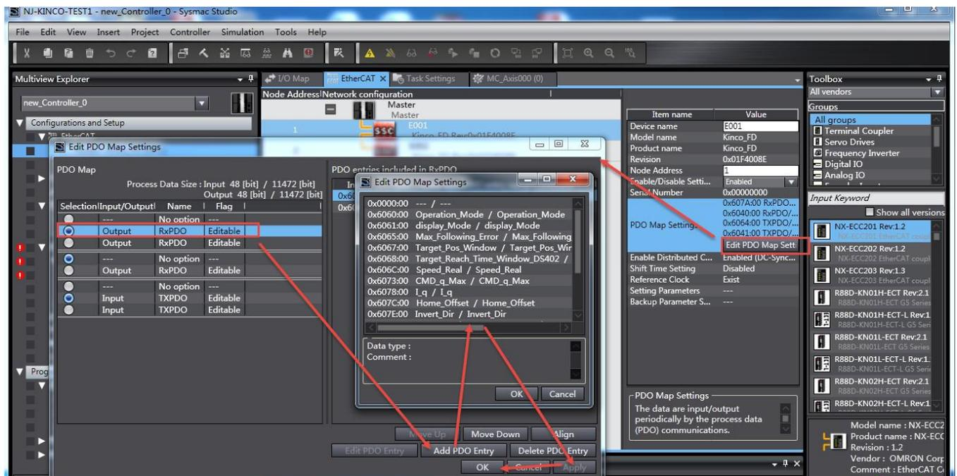
Map slave station' s PDO to controller' s local IO: double click I/O Map at left side and then choose a slave station (the stations have to be configured one by one and all stations must be configured) to crate device variable. The system will distribute a local variable IO automatically.
