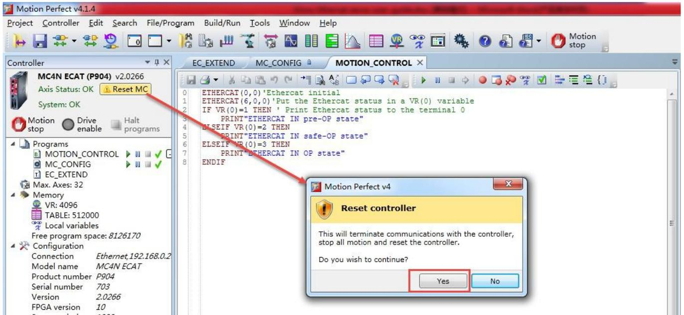
After successful reset, the frame like below (it needs 2min at least for this controller when reset and power on). At the middle area, it is project information file. At left side, it shows the status of controller and slave driver. At right side, it shows the information in window channel 0 that the Ethercat initial program has been executed successfully and the system has found Kinco FD slave which is in Ethercat OP state (Operation state) also.
