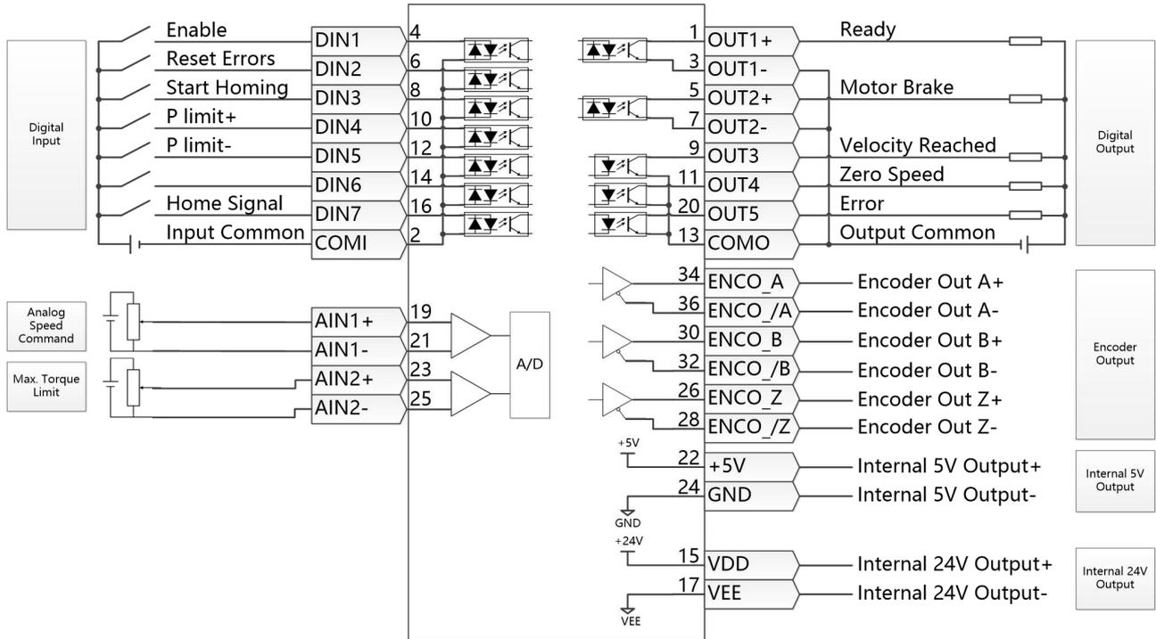
Figure 4-5: X4 wiring in analog control mode
