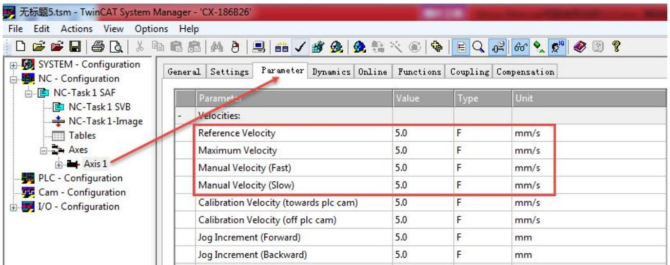
As the shown above, setting speed to 5.0mm/s, then the speed of servo should be  $5.0/0.0001=50000\text{inc/S}=300\text{RPM}$ .
