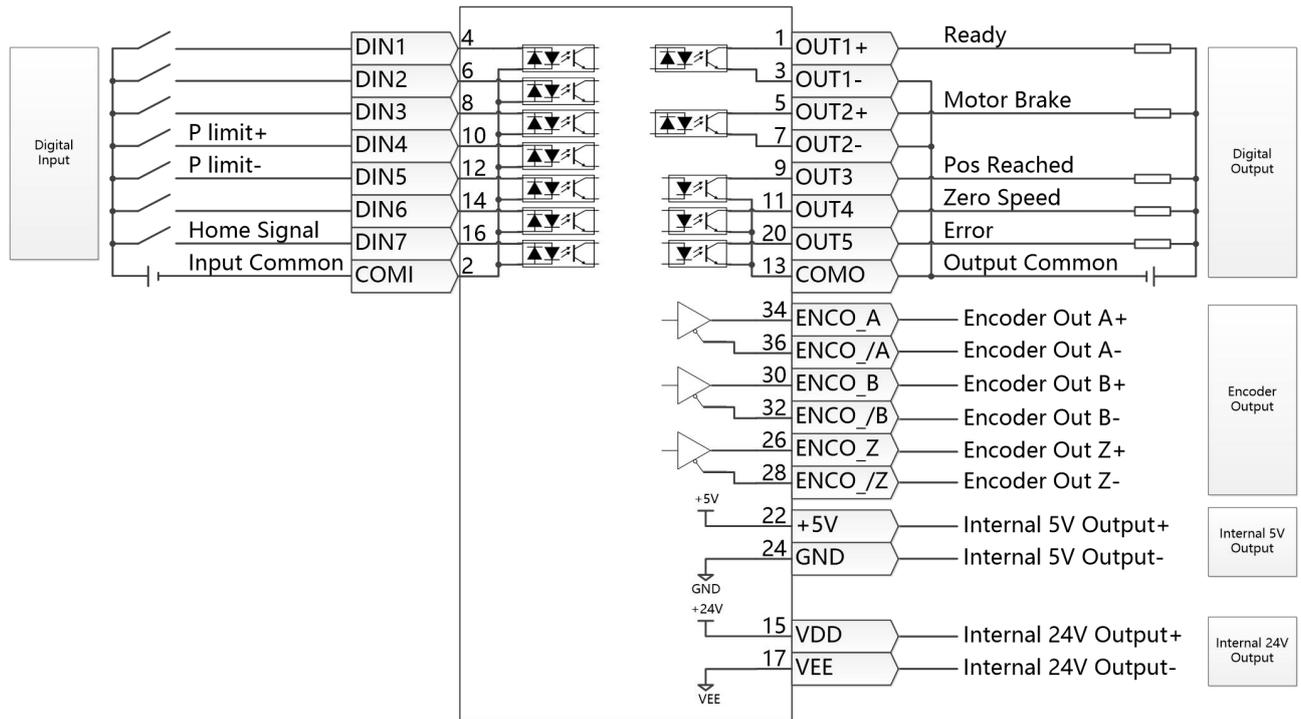
Figure 4-7: X4 wiring in RS232 control mode
