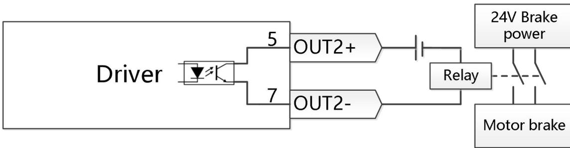
Figure 3-10 OUT2 external relay driver motor lock brake
