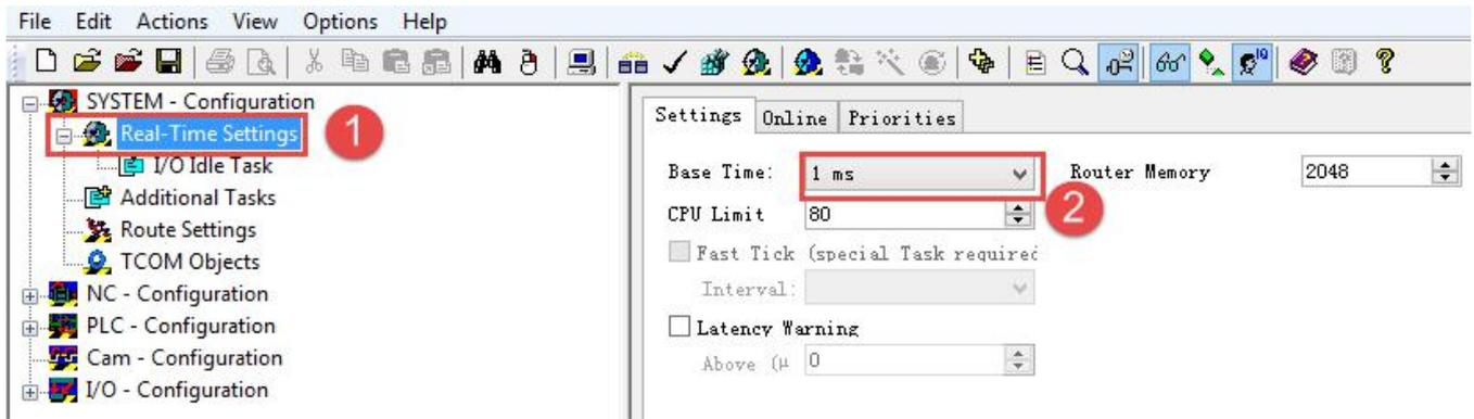
Set NC PTP control period. Generally speaking, the NC period is NC Task SAF period. Here, it is set to 1ms. At this part, TwinCAT NC is used to calculate position, speed and acceleration speed and select direction.
